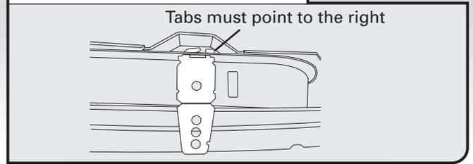
2. Insert the bracket into the slot on the collar. Using a pair of pliers, bend the tab down to secure the bracket in place. Repeat this step for the other side.
